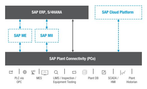
With PCo you can receive tags and events from the connected source systems in the production automatically or on request and transfer them to the connected SAP systems. The component Plant Connectivity offers you the following advantages:
